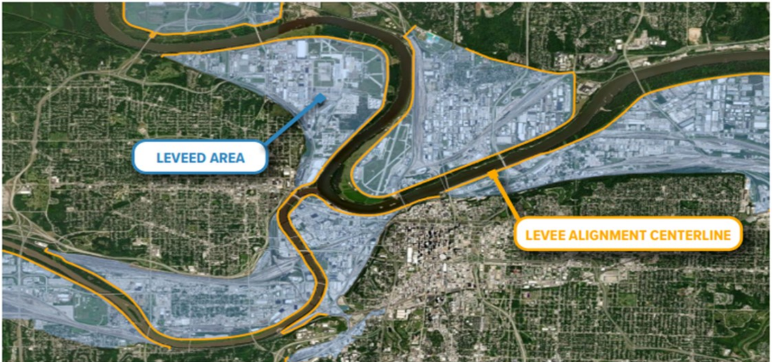
Pictured above: Example levee systems from the National Levee Database showing levee alignment centerlines and leveed areas used for Risk Rating
